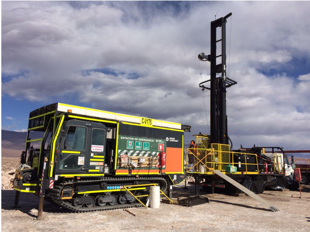
Figure 2: Sonic drill rig onsite at Maricunga lithium brine project.
