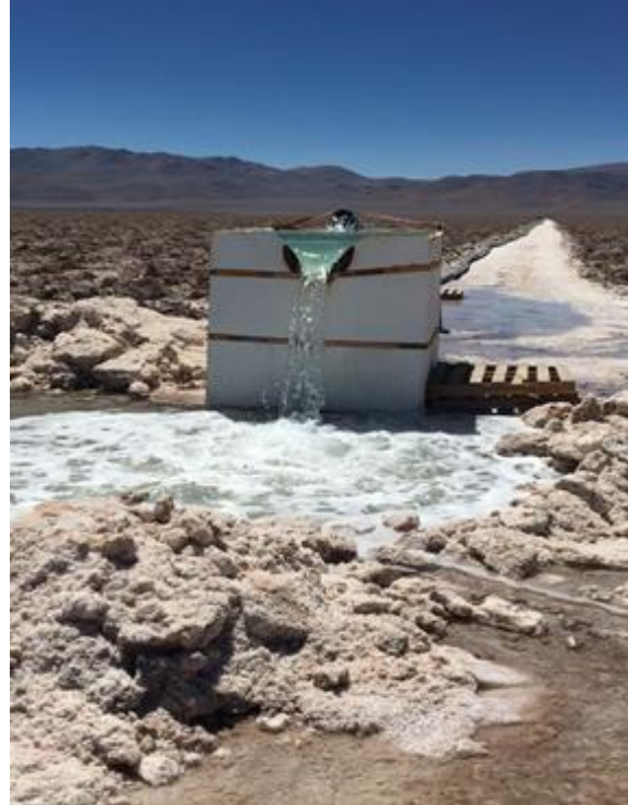
Figure 5: P4 pump test underway
