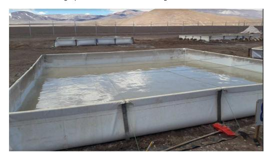
It was evident that the reduction process will be driven not only by solar evaporation but also by wind evaporation as winds were quite gusty at times on site.
